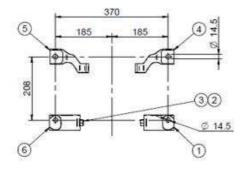
Repowering from Yanmar 1GM10 to Solé Diesel MINI-17 with Supports Pack 370x208 MINI-17 Ref. 13810097
